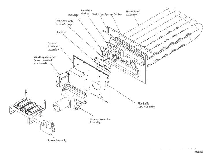
Fig. 31 - Heat Exchanger Assembly
